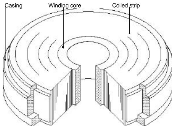
Fig. 2 Layout of STRECON® prestressed container
