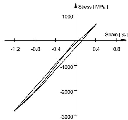
Fig. 9b Tangential stress-strain relation along the critical edge of STRECON® tool
