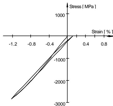
Fig. 9c Tangential stress-strain relation along the critical edge of STRECON® E+ tool
