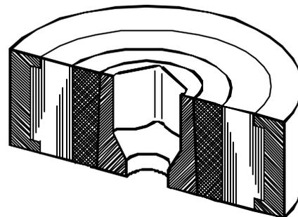
Fig. 3 Layout of STRECON® E<sup>+</sup> prestressed container for manufacture of geometrically complex parts
