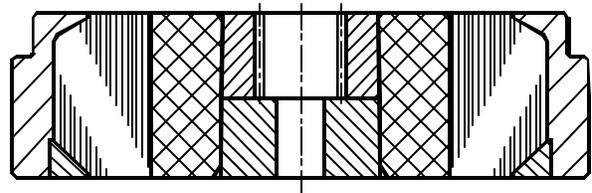
Fig. 11 STRECON® E+ tool for manufacture of planetary gear wheel
