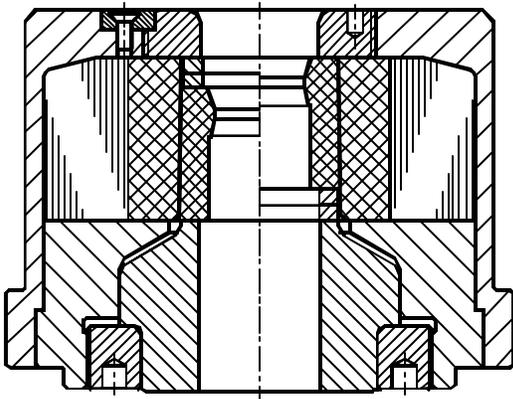
Fig. 13 STRECON® VARI-FIT prestressed container
