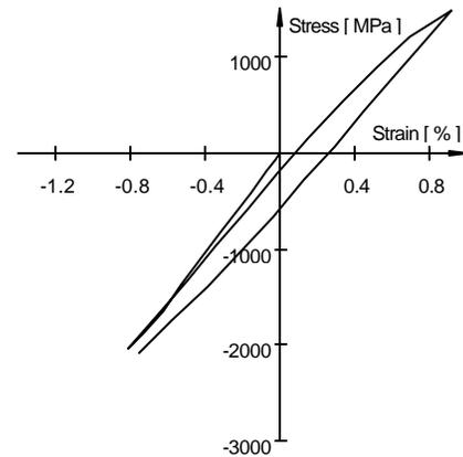
Fig. 9a Tangential stress-strain relation along the critical edge of conventional tool
