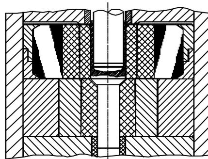
Fig. 4 Tool for manufacture of hollow shaft
