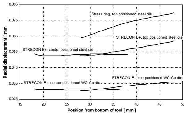
Fig. 12 Die deflections during cold forging of planetary gear wheel
