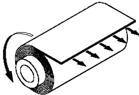
Fig. 1 Winding principle of STRECON® prestressed container
