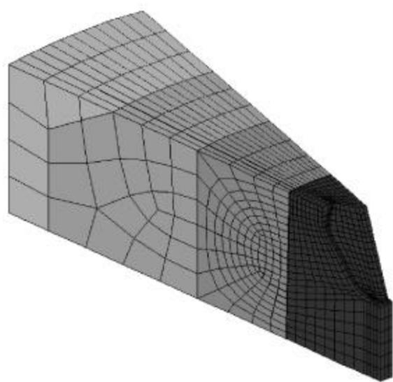
Fig. 7 Finite-element model of STRECON<sup>®</sup> E<sup>+</sup> tool for bevel gear
