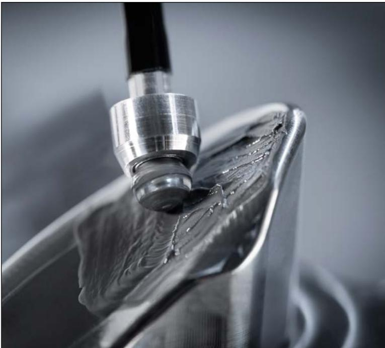
Ball polishing of double-curved mold surface
