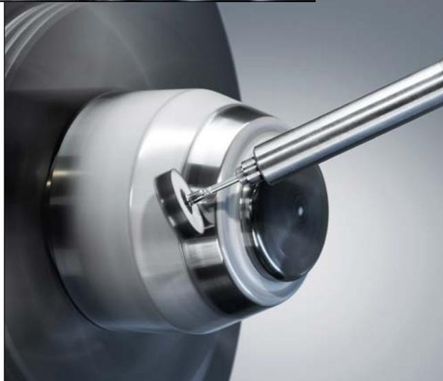
Polishing of a metal forming punch
