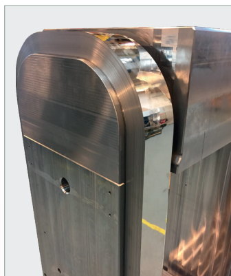
Stripwound press frame construction
