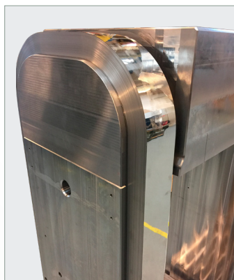
Stripwound press frame construction
