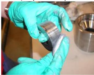
! Excessive lubrication may cause the die to shoot out!
