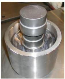
! If the die is divided into **two or more inserts**, they **must be pressed in together**. Otherwise, the insert may shoot out, or the inner bore may get damaged by an uneven press fit.
