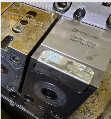
Complete die block design for Hatebur AKP; also applicable for similar machine designs
