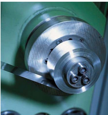
The stripwinding process
