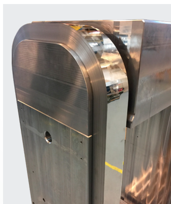
Stripwound press frame construction
