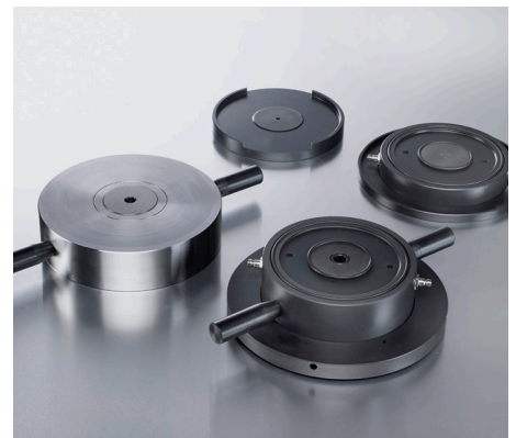
HP-vessel, here shown with quick-connecting external cooling rings
