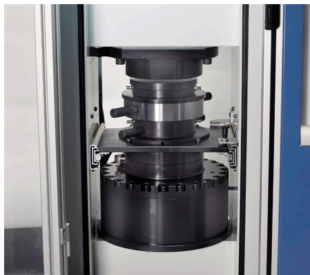
The HP-vessel positioned in the press
