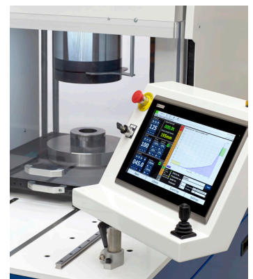
Control panel and sliding press table for proper positioning and setting of the tools
