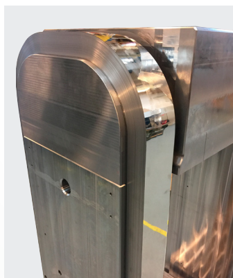
Stripwound press frame construction
