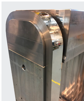
Stripwound press frame construction
