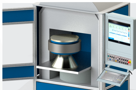
The HP vessel positioned in the press on a sliding table
