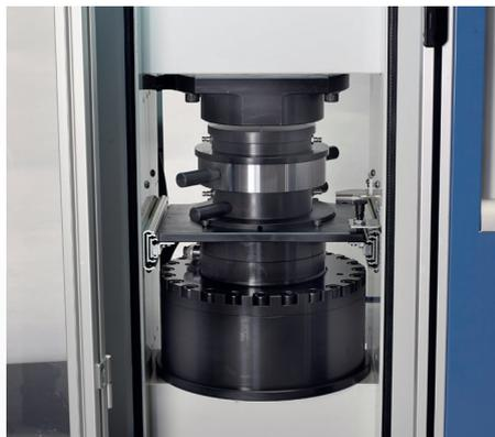
*The vessel positioned in the press*
